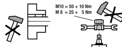
Sealing faces must not be damaged.
